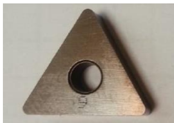
Fig. 1. IS9 \text{Si}_3\text{N}_4 -based cutting insert before ion implantation
